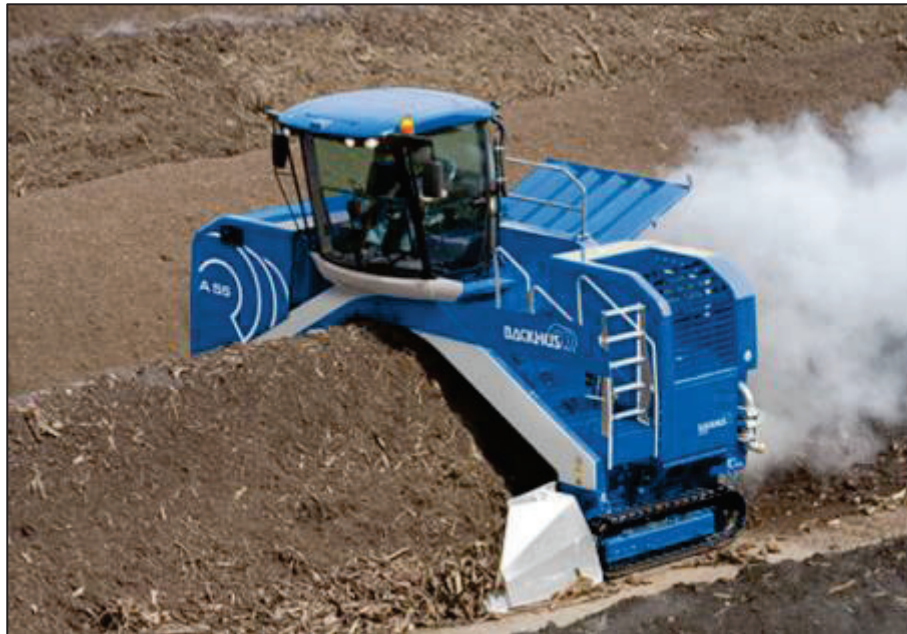
Figure 4.9 Open windrow turner and piles
