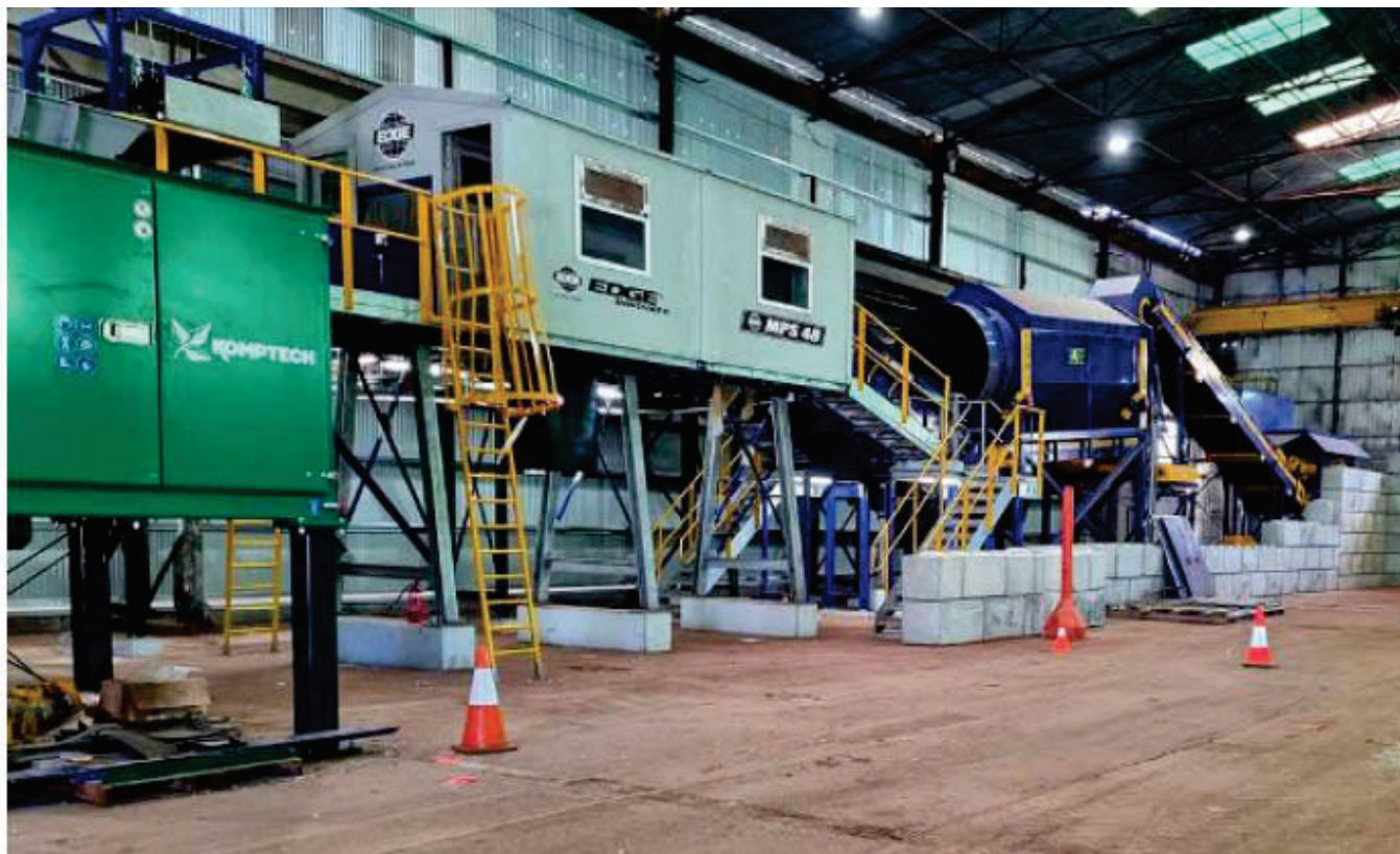
Figure 4.2 Example of sorting, shredding and screening equipment for decontamination and size reduction of material prior to composting
