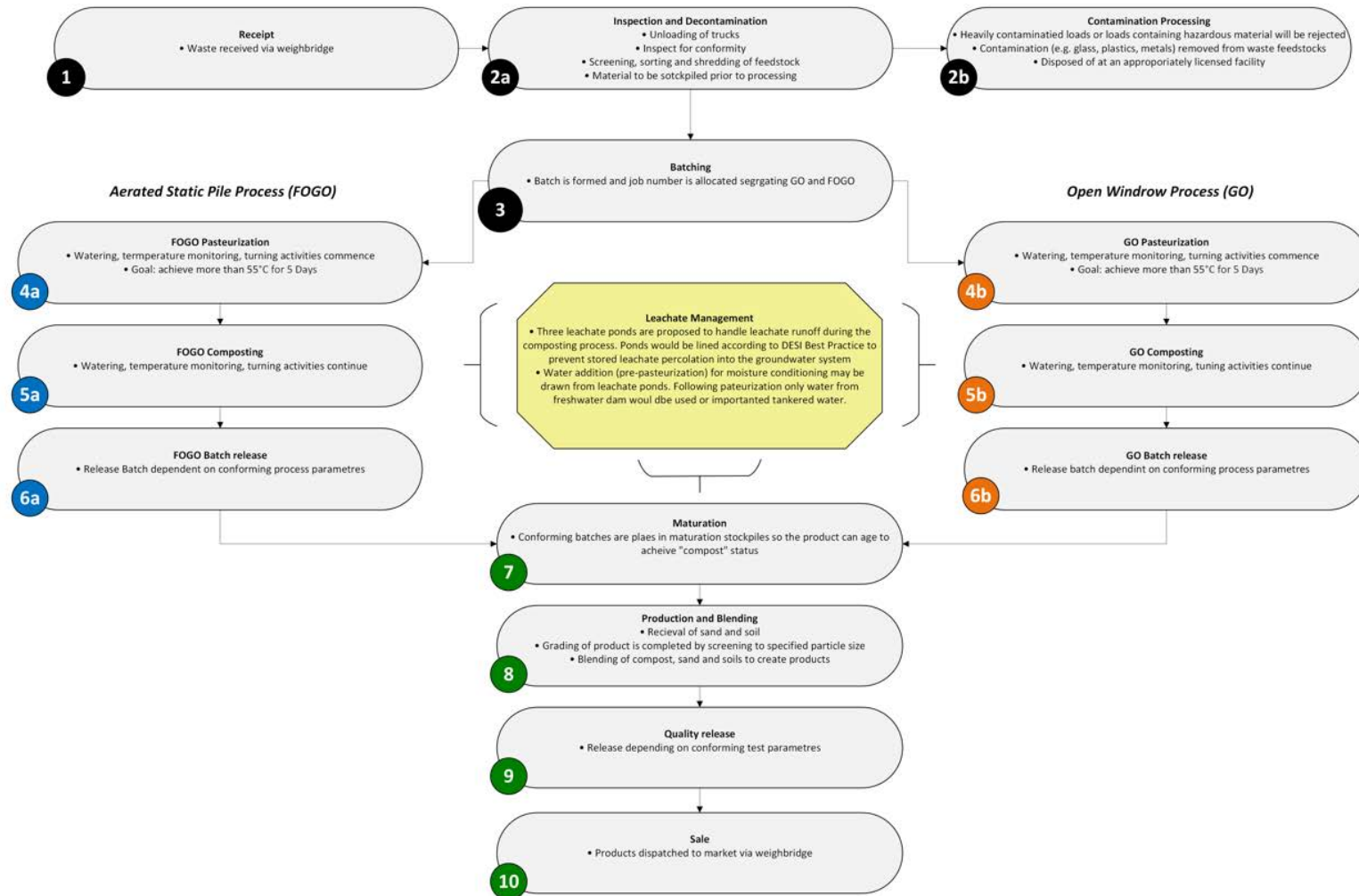
Figure 3 The compost manufacturing process proposed for Bromelton Compost Manufacturing Facility
