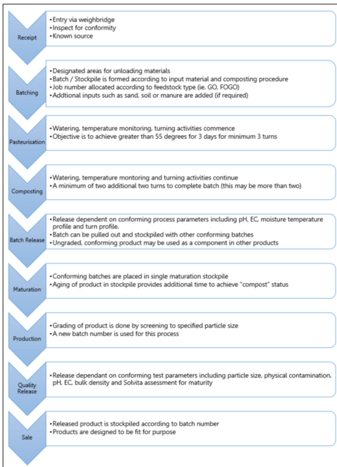
Figure 2-3: Proposed composting process
